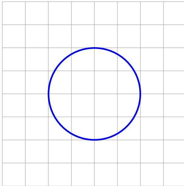
The circle is visible from above. Dividing the 40 m diameter by 10 works out that the diameter on the drawing will be 4 cm. Dividing this by 2 works out that the radius of the circle on the drawing will be 2 cm. Using a compass, drawing a circle with radius 2 cm
