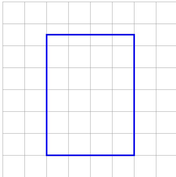
A rectangle is visible from the front elevation. Dividing both the length and width by 10 works out how many centimetres should be drawn for the length and width.  $55 \div 10 = 5.5$  and  $40 \div 10 = 4$
